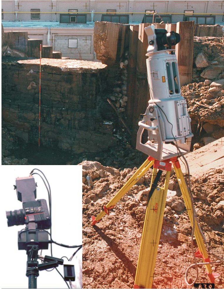
Figure 9 2003–04/Stanhope, New Jersey. The Riegl true-color LIDAR ‘laser radar’ system at Furnace Falls Dam, shown with integrated, high resolution (6 Mp) digital camera (released only in Summer 2003). This system was deployed for the first time in archaeology to capture a high-resolution (mm-precise), 3D record of a flood-damaged historic site. Single-camera photogrammetry, with Rolleimetric camera and software system (inset), was used in tandem with the LIDAR to record, remotely, difficult-to-access or dangerous archaeological contexts. Real-time datum control and reference targets were provided by (1) independent computer transit, total-station system; and (2) on-site, sub-decimeter, dual calibration GPS; these systems were used to geo-reference the LIDAR scans with real-world coordinates of the site grid (Nad83). © 2007 Joel W. Grossman, PhD. Published by Elsevier Inc. All rights reserved.
